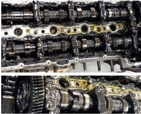
< Contaminated and gelled engine oil >
