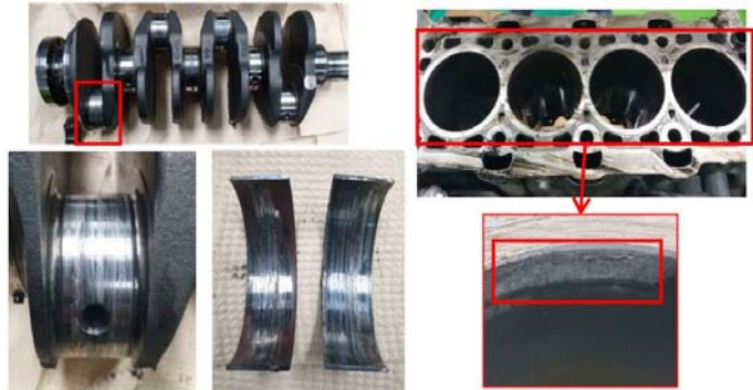
< Excessive wear of moving parts >
